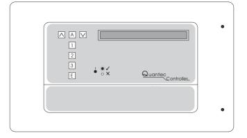
Programming is usually carried out via a laptop PC running Quantec's upload/download PC software (part no. QT707). The buttons on the controller's front can also be used for programming but as this is very time consuming we recommend it for updating existing site data only.
