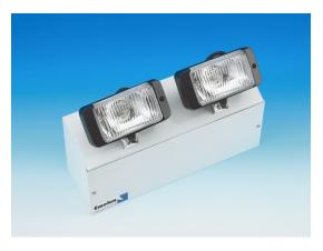
The Premier *ET20* twin projector units provide excellent emergency lighting illuminance for areas requiring high mounting positions. These low cost products utilize twin 20Watt tungsten lamps in adjustable projector heads mounted on a white epoxy coated steel enclosure. The *ET20* twin projector units house 12Volt, five year life Valve Regulated Lead Acid batteries and a high quality charge circuit.
