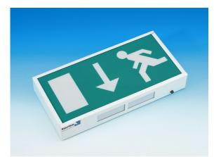
The PF/ES8 range offers a cost effective method of providing statutory safety signs with 3hour duration integral emergency lighting illumination via an 8 Watt T5 lamp. The white epoxy coated steel base and screen printed polycarbonate legend panel enclose a removable gear tray. The *ES8* exit signs are easy to install and are supplied with appropriate legends complying with the Health and Safety (Signs & Signals) Regulations.
