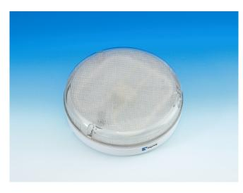
The Premier *EL2D* range of luminaires offers a cost effective method of providing mains lighting or emergency lighting in areas requiring attractive but robust IP65 rated luminaires. The polycarbonate base and diffuser house a removable gear tray, control gear and **28Watt 2D** lamp. The luminaires are provided with side and back conduit entries and are easy to install.
