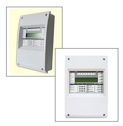
The panel is equipped with a backlit LCD display of 4 rows each with 40 characters to give clear textual indications of Fire / Fault occurrences to the end user. Additionally mini-repeaters can be connected via an RS422/RS485, Fibre Optic or TCP/IP interface to facilitate remote display and control of the system.
